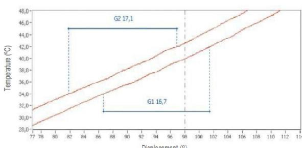
Perfect sensitivity with a long distance during temperature from 34 to 42 degrees adjustments. Easy to adjust the temperature and get the right temperature for shower/washing (Norm EN-817; Norm NF-077).
