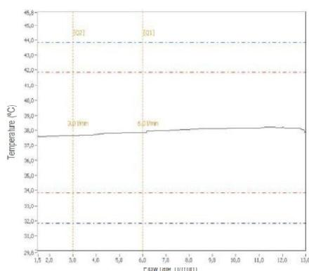
Constancy of temperature: the design of ceramic cartridges provides a constancy of temperature at any flow adjustment and allows the user to maintain the same temperature (Norm NF-077)
