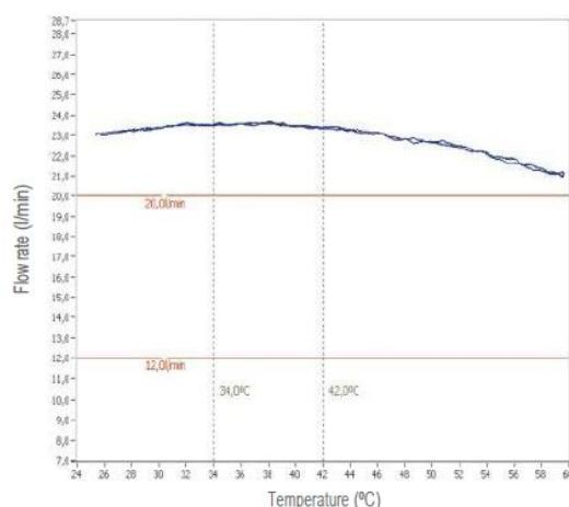
Flow rate: a high flow rate provides the tap manufacturers an easy adjustment, obtaining the desired flow by easily adjusting the aerators. This allows different flows depending on customers design characteristics.
