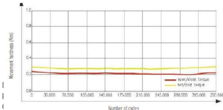
Service life to minimum 70,000 cycle according the norm EN-817 / NF-077, minimum 350,000
